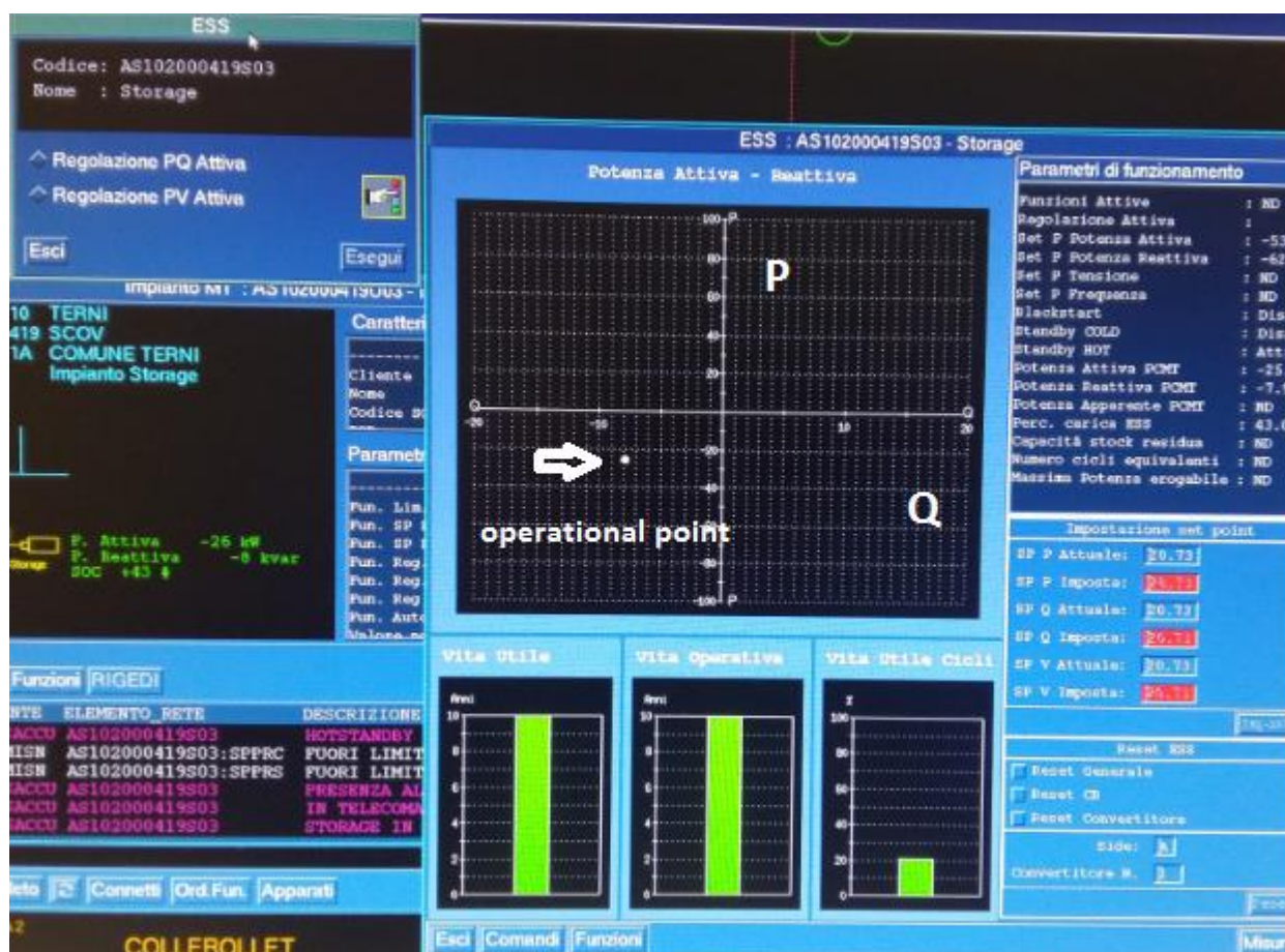
Figure 10: SCADA HMI interface during a (P,Q) request
